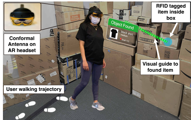
Figure 1: X-AR enable its user to see and locate hidden items in the environment by fusing AR and RF sensing.
